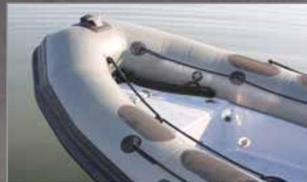
**IMPACT COLLARS AFFORD SHOCK ABSORPTION AND FACILITATE BOARDINGS. BCGP'S POLYURETHANE MATERIAL HAS FOUR TIMES THE ABRASION RESISTANCE OF HYPALON OR PVC.**
